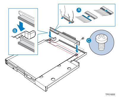
Figure 22. Installing the Floppy Drive Interposer Board
